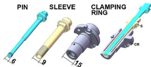
Figure 1: Schematic illustration of FSpJ tool comprised of a pin, sleeve and clamping ring (dimensions are in mm).
