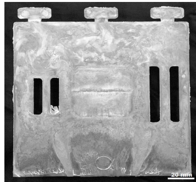
Fig. 2. MRI230D cast at a die temperature of 180°C and a high speed plunger velocity of 1.3 m/s showing spangled surface. This is the worst case observed.
