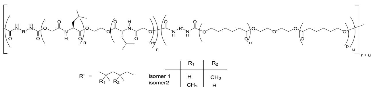
**Scheme 1.** Multiblock copolymer PCL-PIBMD, which were prepared using TMDI (2,2,4 and 2,4,4 isomers) to build up junction units
