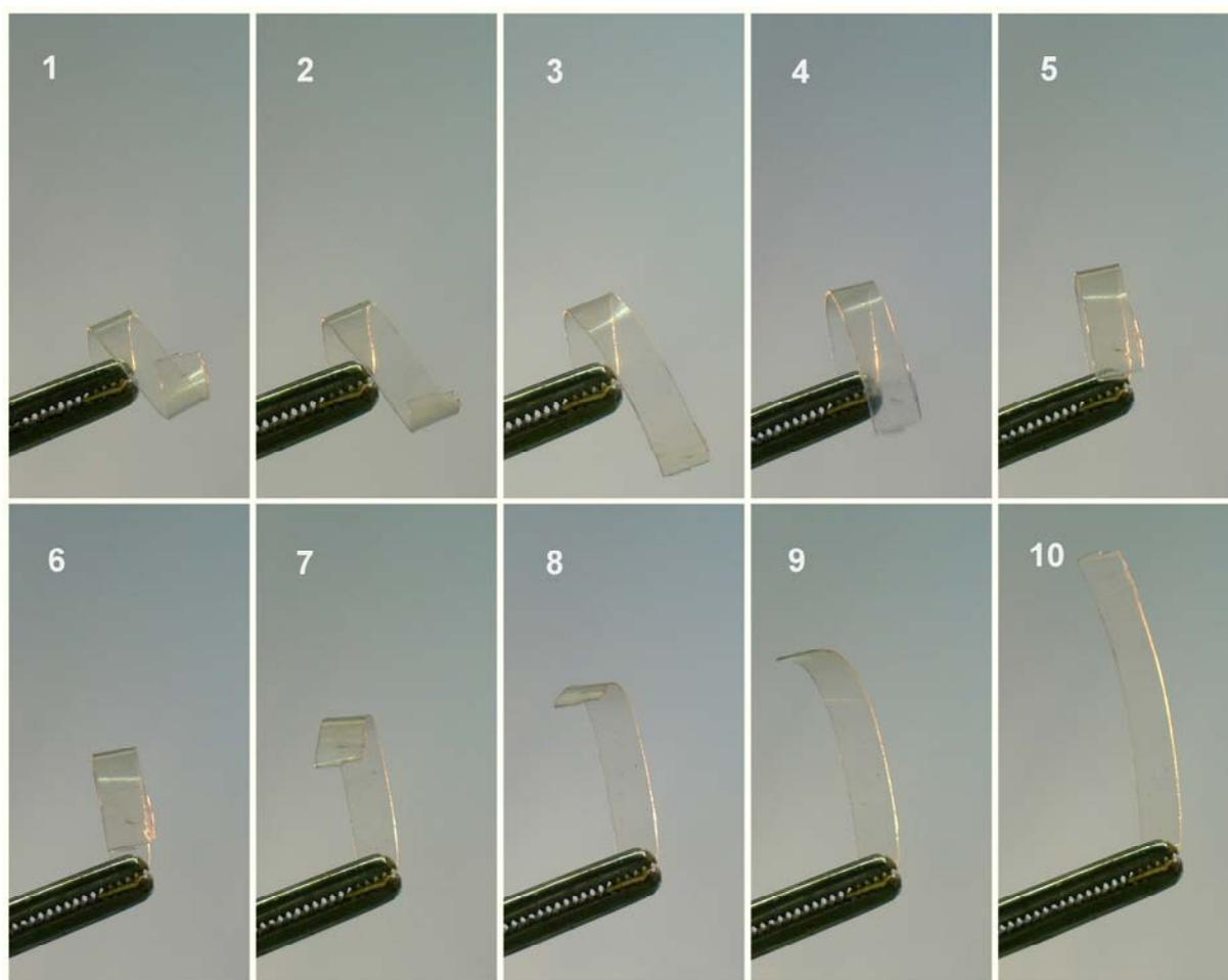
**Figure 1.** The series of photographs (1-10) demonstrates the macroscopic shape-memory effect for PCL-PIBMD50. The transition from the temporary shape (“corkscrew”, 1) to the permanent shape (“stripe” 10) took approx. 30 s at  $60 \text{ }^\circ\text{C}$ .
