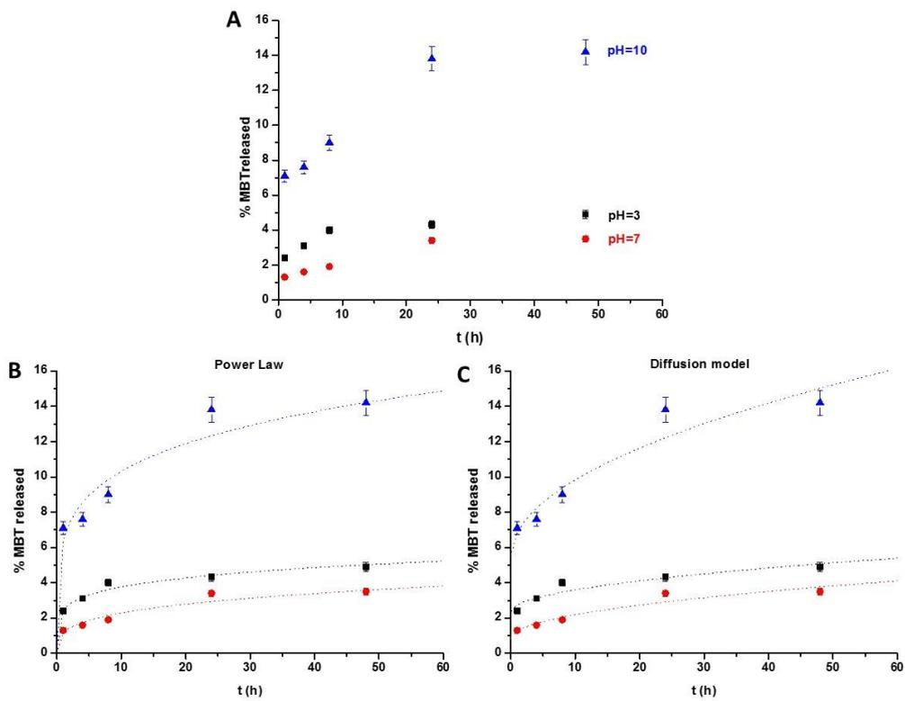
Figure 3: (A) Release profiles of MBT from MBT@PU-MC in different pH conditions. Fittings of experimental data using different kinetic models: (B) Power Law and (C) Higuchi's square root of time (diffusion model).
