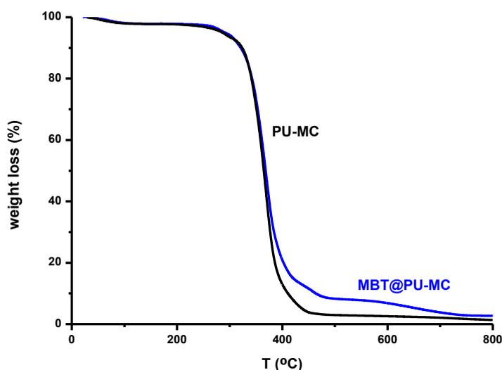
Figure 2: TG profiles of empty PU-MC and MBT@PU-MC
