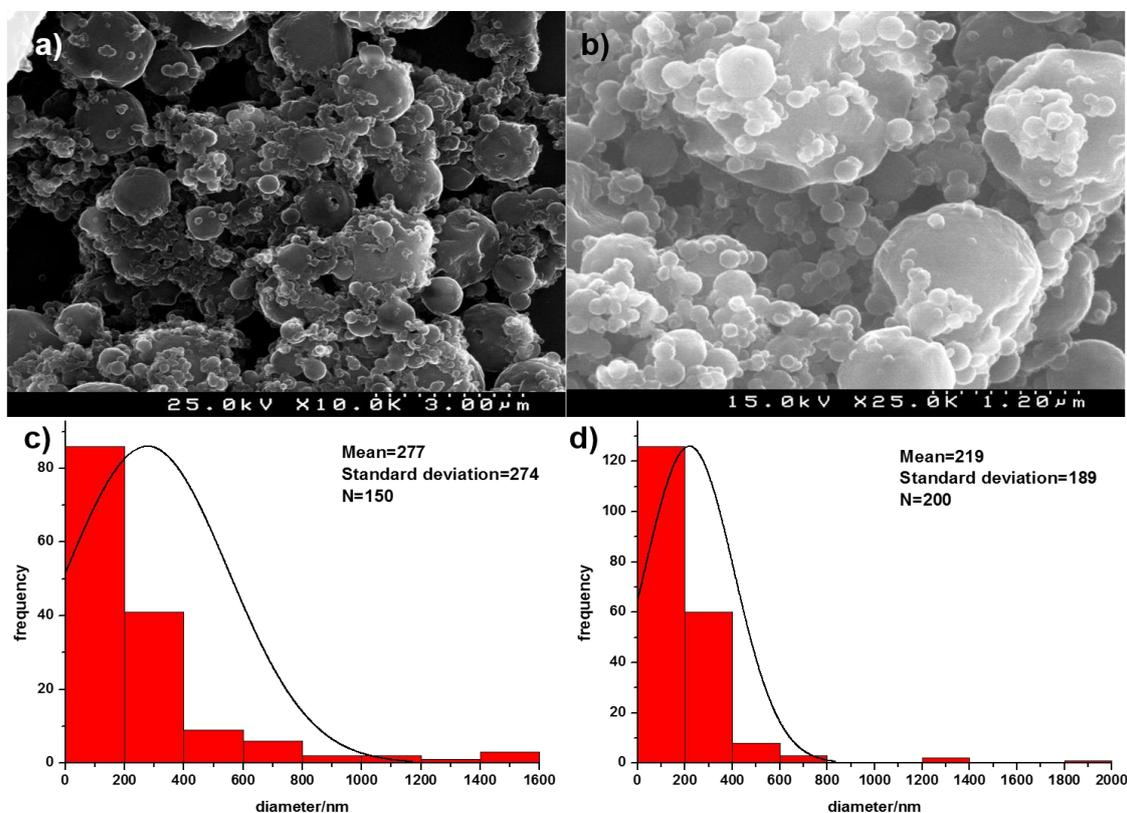
Figure 1: SEM images of (a) empty PU-MC, (b) MBT@PU-MC; Size distribution histograms of (c) empty PU-MC and (d) MBT@PU-MC.
