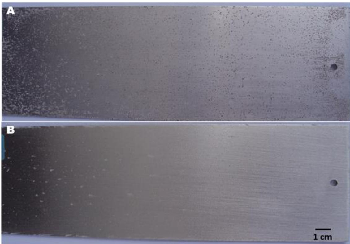
Figure 8: Coated AA2024 with (A) unmodified sol-gel and (B) with sol-gel containing MBT@PU-MC, after 168 hours in NSS.
