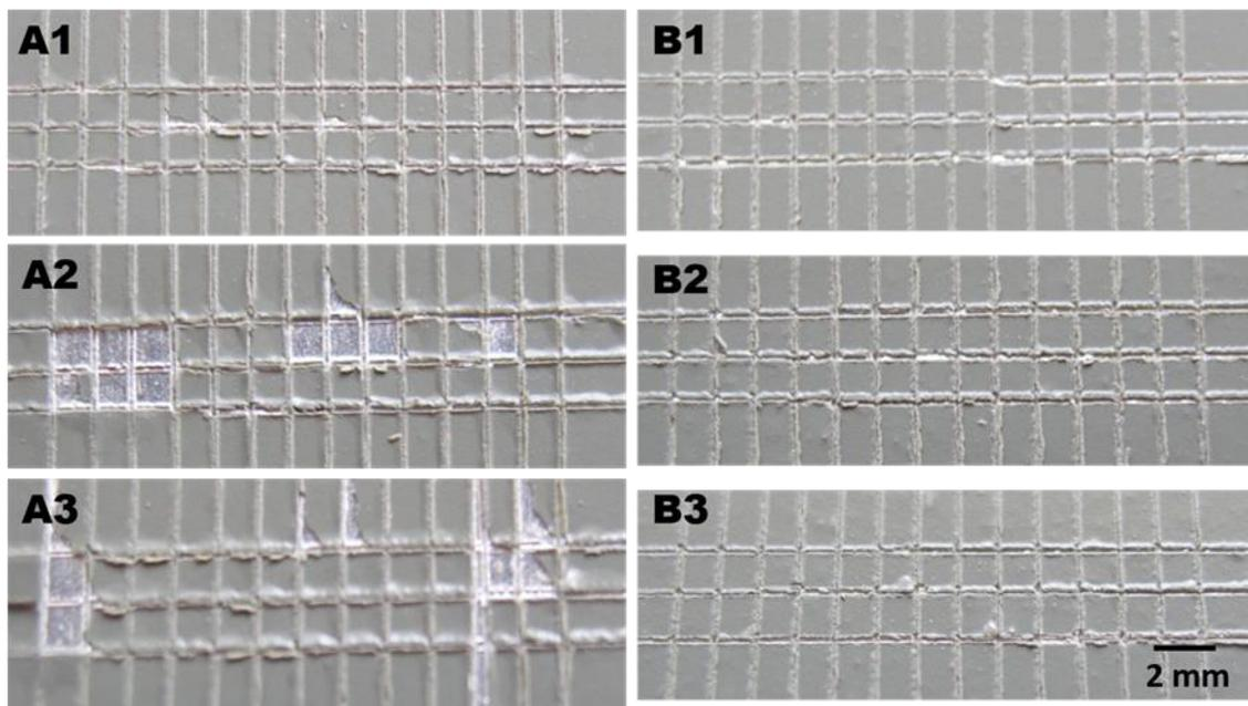
Figure 9: Coated AA2024 with (A) unmodified sol-gel + primer/top and (B) modified sol-gel with MBT@PU-MC + primer/top, after cross-cut test.
