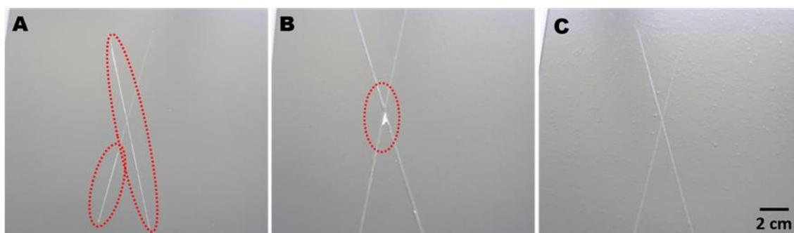
Figure 10: Coated AA2024 with (A) primer/top, (B) unmodified sol-gel + primer/top and (C) sol-gel with MBT@PU-MC + primer/top, after wet x-cut test.
