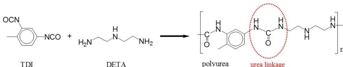
Scheme 1: Reaction of the amine groups of DETA with isocyanate group of TDI forming the urea linkage.
