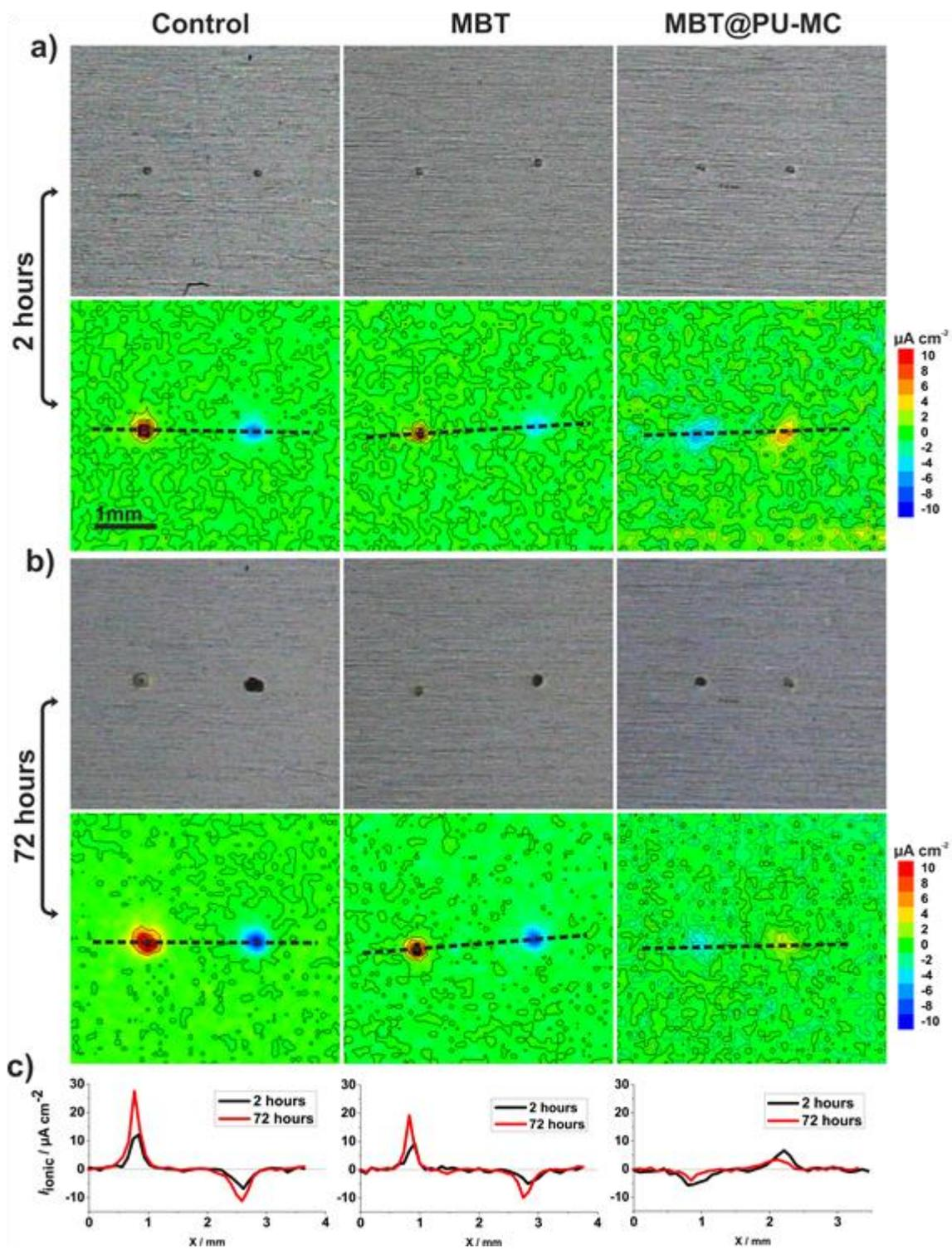
Figure 7: Optical micrographs and SVET maps after 2 hours of immersion (a) and after 72 hours of immersion in 0.05M NaCl (b) and selected ionic current profiles (c) for all samples.
