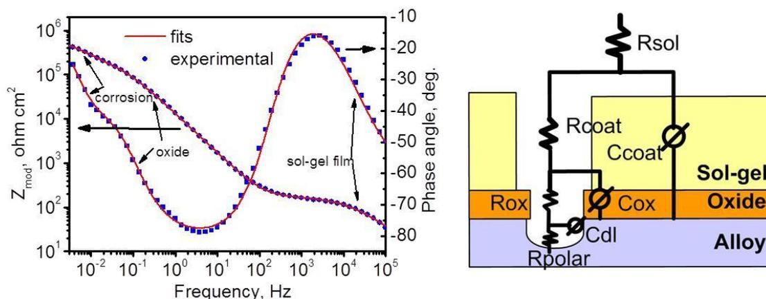
Figure 5: Schematic representation of EIS fitted data (left) using equivalent circuits model (right). Adapted from [37].
