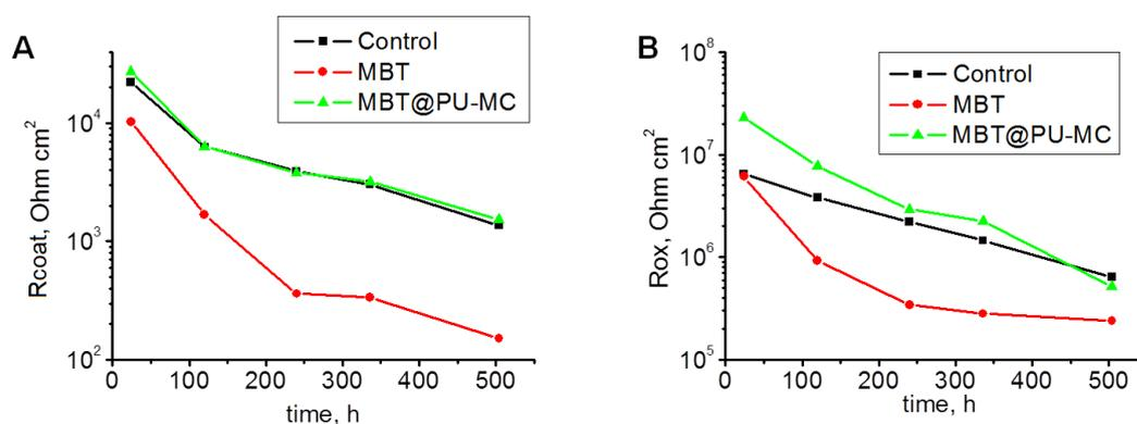
Figure 6: Evolution of sol-gel film resistance (A) and intermediate oxide layer resistance (B) for samples with unmodified sol-gel, sol-gel with MBT and MBT@PU-MC during immersion in 0.5 M NaCl.
