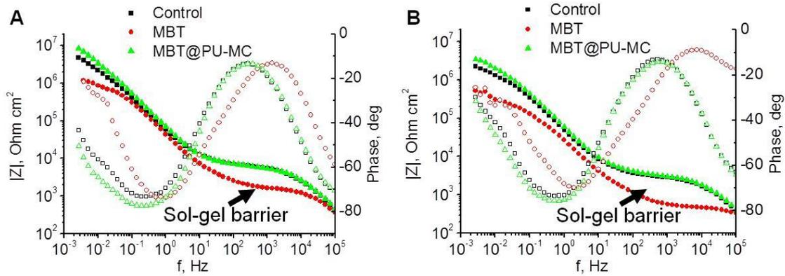
Figure 4: Bode plots of coated AA2024 immersed in 0.5M NaCl solution after (A) 5 days and (B) 14 days.
