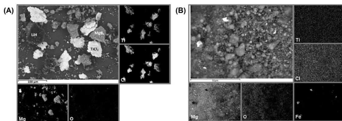
Figure 4: SEM images in backscattering and EDS modes (A) unmilled sample (B) and a 30 h milled sample, with elemental distribution of Mg, Ti, Cl, O and Fe.
