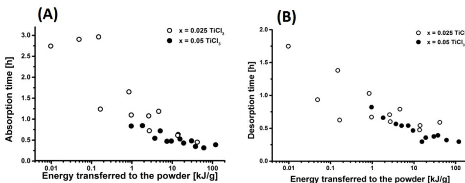
Figure 1: (A) Absorption and (B) desorption times shown as a function of the calculated energy transferred to the powder during the milling process.
