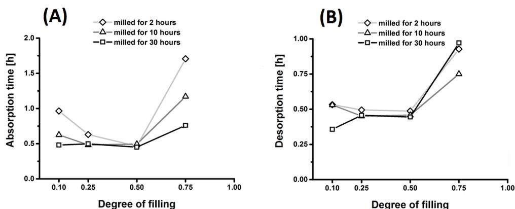
Figure 3: (A) Absorption and (B) desorption time with respect to energy transferred from the milling process to the powder.
