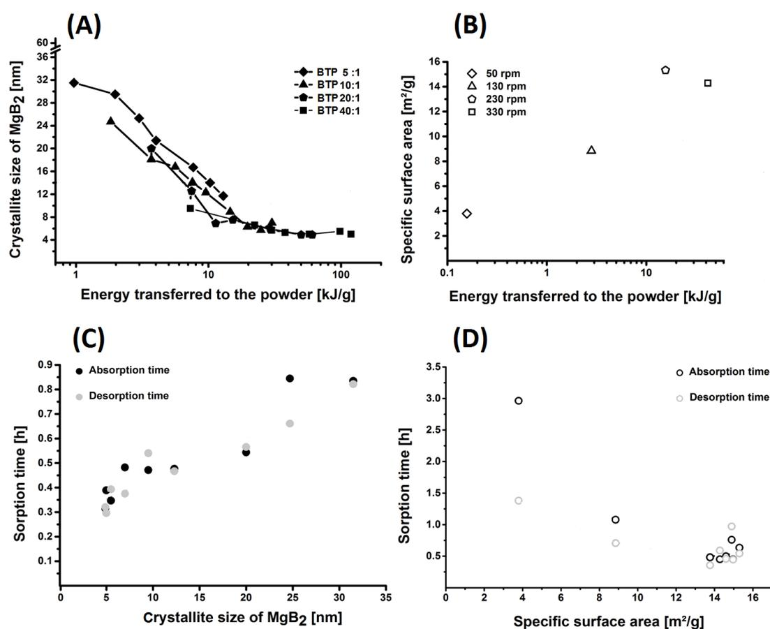
Figure 2: (A) Crystallite size of  $MgB_2$  and (B) specific surface area as a function of the energy transferred to the powder. Sorption times changes with (C) crystallite size of  $MgB_2$  and (D) specific surface area.
