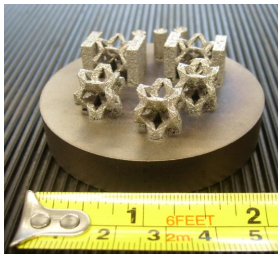
Figure 12: Produced TNMB1 3D-dodecahedron structures with optimized parameter set
