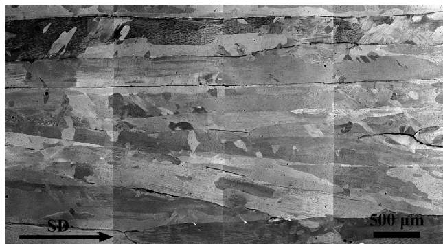
FIG. 1. Microstructure of directionally solidified and homogenized alloy at room temperature, showing the columnar-shaped morphology of original austenite grains.
