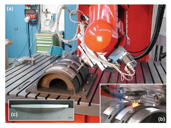
Fig. 54. FS of stainless Steel on a mild steel cylindrical partusing a Tricept TR805 robot. (a) Setup and clamping system, (b) deposition, (c) cross section macrograph of coating (Beyer et al., 2003).
