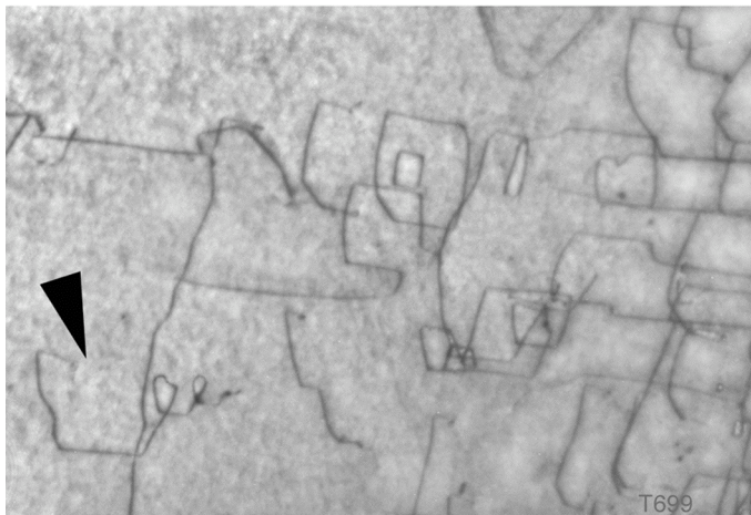
Fig. 7. Defect recovery during in situ heating inside the TEM. Note the growth of the debris defects, the generation of a new loop (arrow 1), presumably due to the aggregation of excess vacancies (arrow 1) and the formation of helical dislocations (arrow 2), because of vacancy absorption. Ti-48Al-2Cr, pre-deformation at room temperature in compression to \epsilon=3\% . Acceleration voltage 120 kV.
