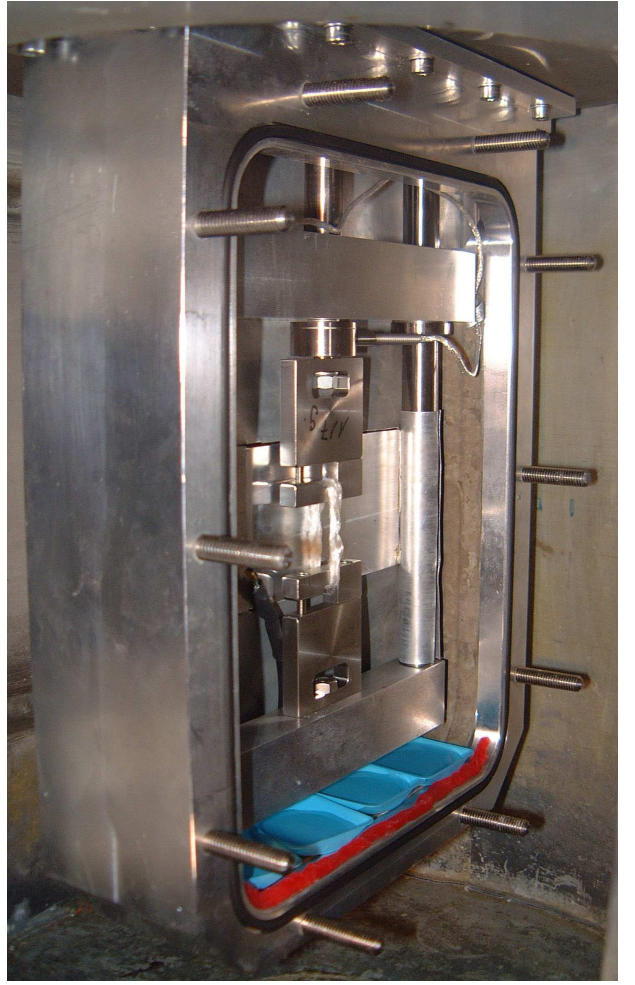
FIG. 1: (color) Photograph of a silk sample (white fiber bundle in the center of the image) inside the humidity chamber for in situ tensile testing mounted inside the sample bay of the time-of-flight spectrometer IN6. The chamber is shown with the front cover removed. The force sensor is visible as a cylindrical metal structure on the upper center of the photograph with the signal cable arriving from the right. The neutron beam impinges on the sample horizontally, arriving from the right edge of the photograph. The blue plastic troughs at the bottom of the chamber contain pure water or saturated salt solutions, respectively, to define the humidity inside the chamber. The edge-to-edge distance between the steel hooks holding the fiber bundle is 3 cm.
