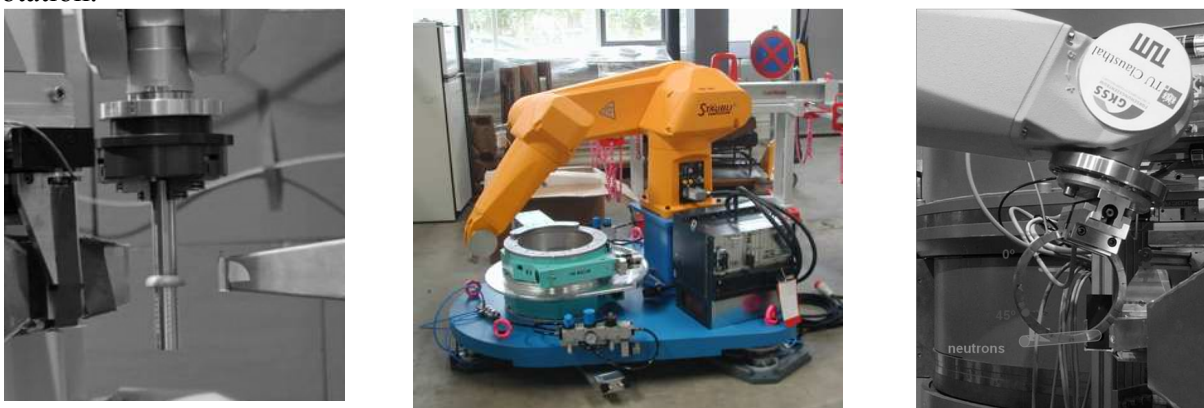
Fig.5: Stäubli RX160 (middle) with mounted samples (friction weld – left; Cu-ring – right)
