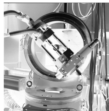
Fig.1b: Loading device with a compression sample mounted in a Eulerian cradle
