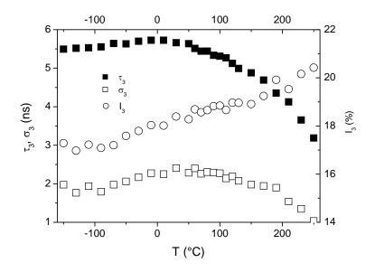
**Figure 3**: Temperature dependence of o-Ps lifetime  $\tau_3$ , dispersion  $\sigma_3$  and Intensity  $I_3$  of PIM1-CO1-40; note the maximum in  $\tau_3$  at approx. 0 °C.
