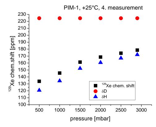
Figure 11: Behaviour of the <sup>129</sup>Xe chemical shift of the Henry and the Langumir sites in PIM-1.
