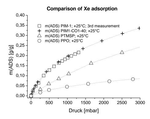
**Figure 6**: Comparison of Xenon sorption curves of PIM-1, PIM1-CO1-40 (both after 100°C Xesorption), PTMSP<sup>60</sup> and PPO at 25°C.<sup>58</sup>
