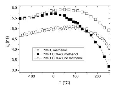
**Figure 4**: Comparison of o-Ps lifetime  $\tau_3$  as function of temperature for PIM-1 and PIM1-CO1-40, both methanol treated to be in a well defined, relaxed state, and the PIM1-CO1-40 also without methanol treatment for comparison.
