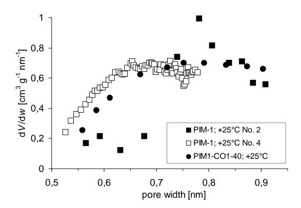
**Figure 7:** Pore width distributions determined by the Horvath-Kawazoe method from Xe adsorption at 25°C for PIM1-CO1-40 ( $\bullet$ ) and for PIM-1 batch CT/02/07 before ( $\blacksquare$ ) and after ( $\Box$ ) Xe adsorption at 100°C.
