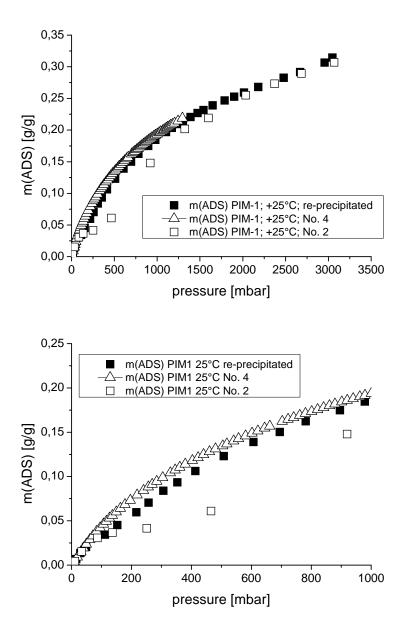
**Figure 5**: Sorption of Xe on PIM-1 at the second  $(\Box)$  and forth  $(\Delta)$  sorption cycle and after re-dissolving in CHCl<sub>3</sub> and re-precipition in MeOH ( $\blacksquare$ ). The numbers given for the specific measurements reflect the sample's thermal history (See Tab. 4).
