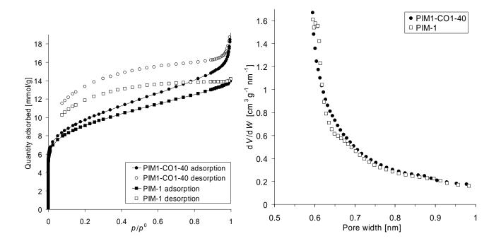
**Figure 2**: (a) N<sub>2</sub> adsorption (filled symbols) and desorption (open symbols) isotherms at  $-196^{\circ}$ C for PIM1-CO1-40 ( $\bullet$ , $\bigcirc$ )and PIM-1 batch CT/02/07 ( $\blacksquare$ , $\Box$ ) and (b) pore width distributions obtained by analysis of N<sub>2</sub> adsorption at  $-196^{\circ}$ C by the Horvath-Kawazoe method.
