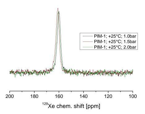
**Figure 9**: <sup>129</sup>Xe NMR spectra of Xe adsorbed on unrelaxed PIM-1 at Xe pressures between 1 and 2 bar over the sample.
