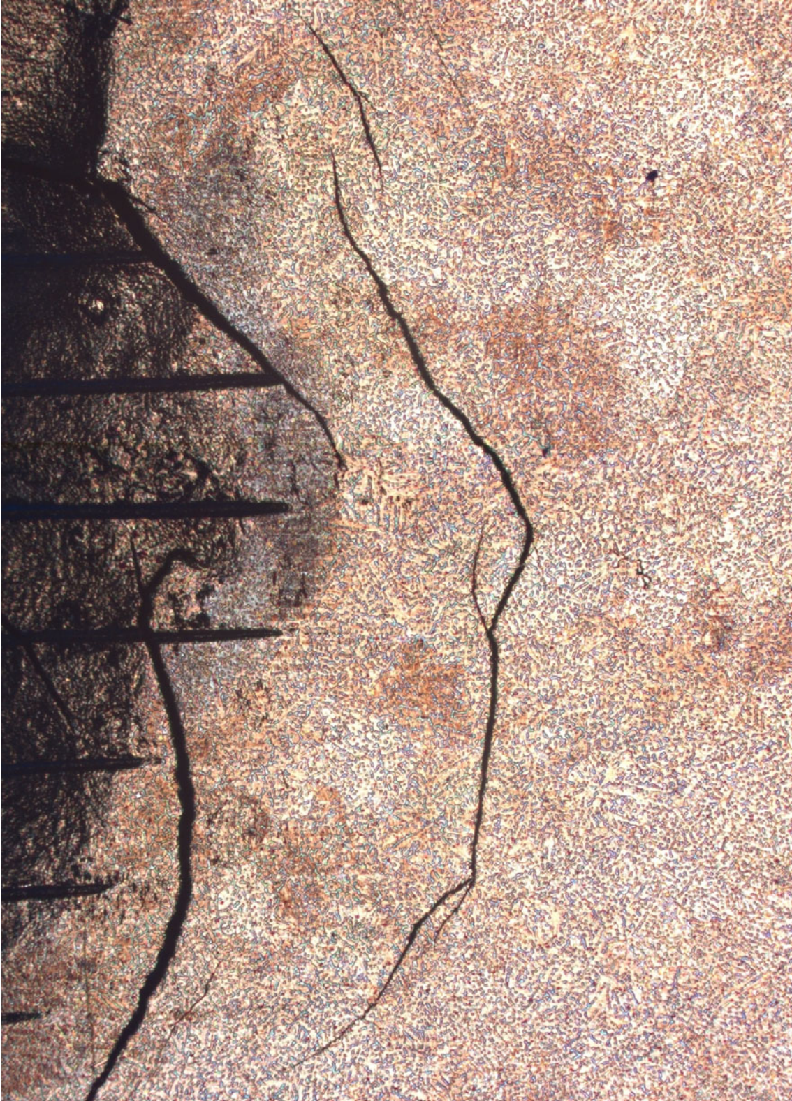
Figure 9 – Surface secondary cracking in AZ91 CT specimen tested in distilled water.
