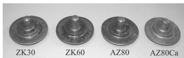
7 Magnesium alloy forgings worked at 350°C after pre-extrusion
