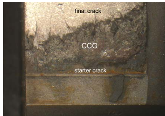
Figure 3 – Fracture surface of a tested CS(T) specimen of BW P22 with starter crack in WM. Sectioned specimen half
