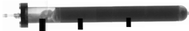
Figure 6: Neutron radiography of NESSHY tank using fission neutrons at the NECTAR beamline of the FRM II facility in Garching, Germany
