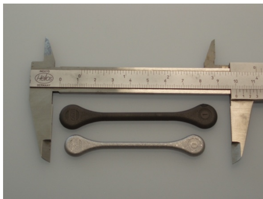
Fig. 2. Injection moulded and the as-sintered “dog-bone” tensile test specimens.
