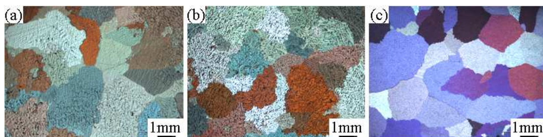
Fig. 3. Optical microstructures of ternary Mg-1.5Zn-xY alloys showing the grains: (a) x=0.2, (b) x=2, (c) x=4.
