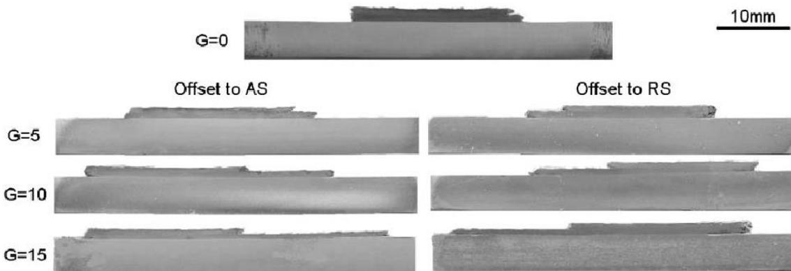
Fig. 40. Macrostructures of multilayer deposit for several overlapping distances. AA5052 over AA2017 (Tokisue et al., 2006).
