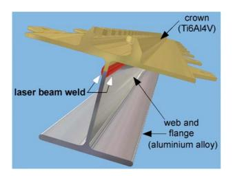
**Fig. 1** The passenger seat track as a laser beam welded dissimilar joint, (conceptual design after AIRBUS. The total height of the assembly is about 61 mm, the web height about 45 mm and the aluminium alloy flange width about 50 mm; drawing not to scale).
