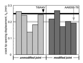
**Fig. 8** Resistance to fracture in terms of crack tip opening displacement, CTOD  $\delta_5$ . The horizontal bands show the base material data for Ti6Al4V and AA6056-T6.
