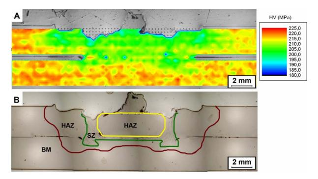
Figure– 3 – (A) Microhardness distribution and (B) Proposed microstructural weld zones of a typical FSp joint on PMMA.
