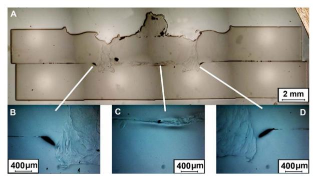
Figure– 2 – Microstructure of a PMMA joint of FSpW ("sleeve plunge" at 500 rpm/ 5.5 s/ 3 bar/ 4 mm ): (A) Cross-sectional view from the weld center; (B) and (D) Details of the consolidated plasticized polymer; and (C) The central region of the spot, showing the bonding line between upper and lower plaques.
