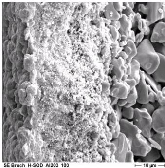
26 **Fig. 3:** SOD membrane layer on top of an  $\alpha$ -Al<sub>2</sub>O<sub>3</sub> support disc
