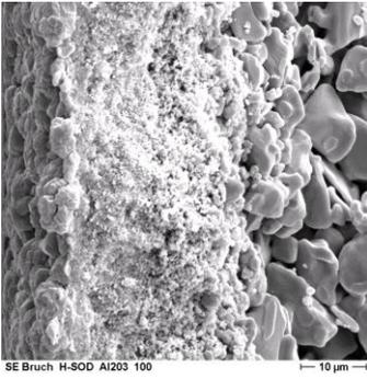
**Fig. 3:** SOD membrane layer on top of an  $\alpha$ -Al<sub>2</sub>O<sub>3</sub> support disc
