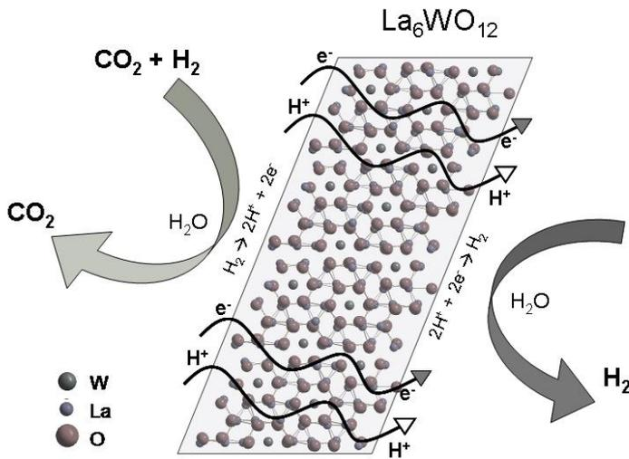
14 **Fig. 5:** Scheme of the permeation process in a mixed protonic-electronic conducting membrane made of  $\text{La}_6\text{WO}_{12}$
