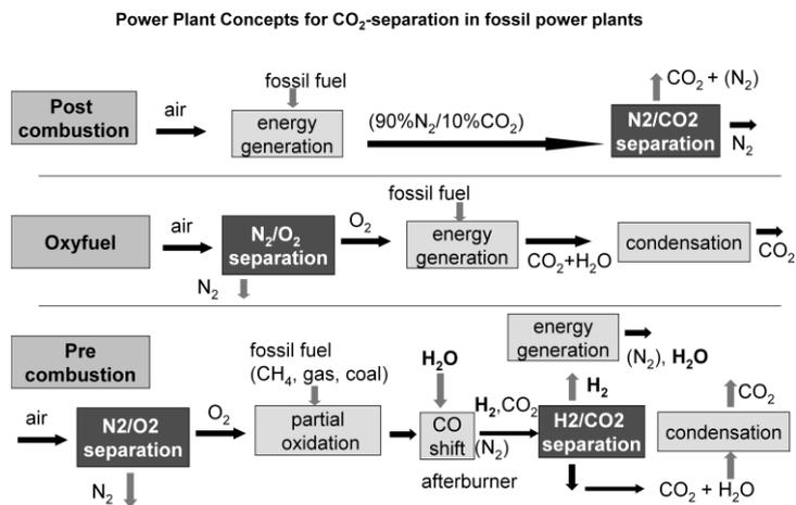
Fig. 1: The three CO<sub>2</sub> capture concepts
