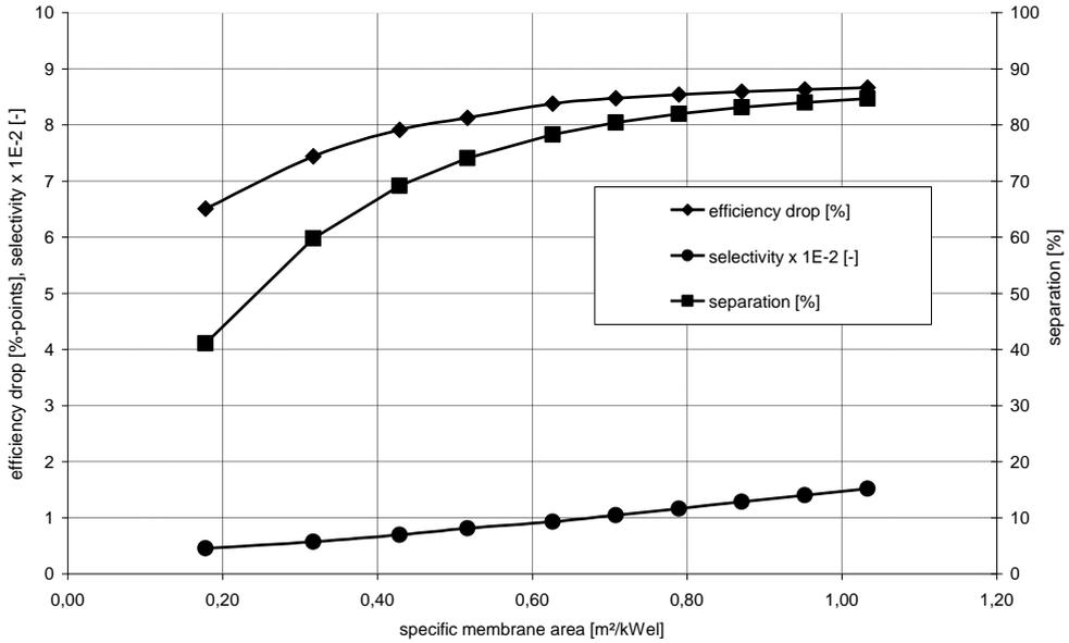
Fig. 8: Results of single membrane concept simulations for the integration of polymeric membranes
