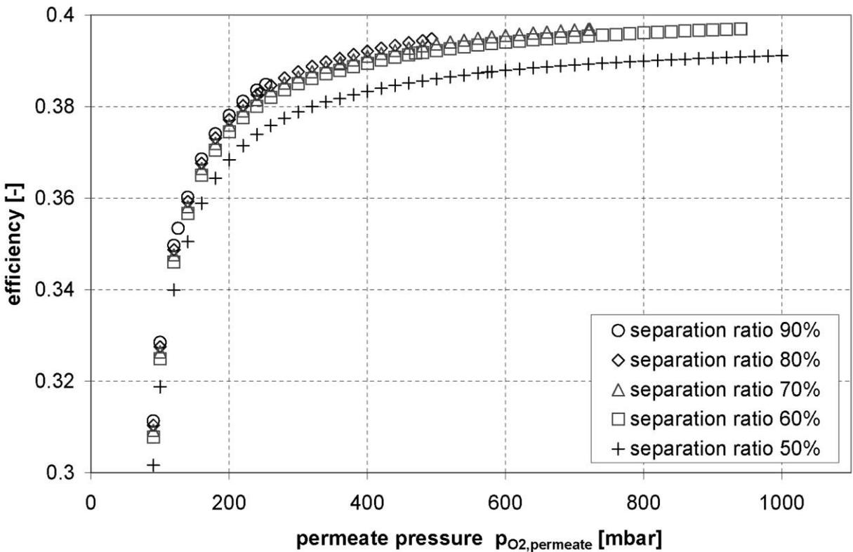
Fig. 9: Influence of the separation ratio and the permeate pressure on the efficiency of an oxyfuel power plant (1210 MW<sub>th</sub>) at 10 bar feed pressure.
