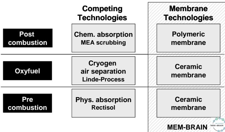
Fig. 12: Comparison of different CCS technologies
