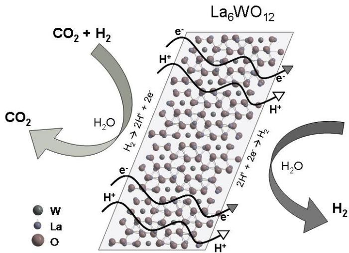
**Fig. 5:** Scheme of the permeation process in a mixed protonic-electronic conducting membrane made of La<sub>6</sub>WO<sub>12</sub>
