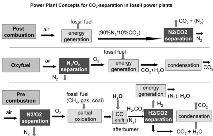
Fig. 1: The three CO<sub>2</sub> capture concepts
