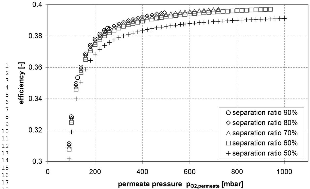
**Fig. 9:** Influence of the separation ratio and the permeate pressure on the efficiency of an oxyfuel power plant (1210 MW<sub>th</sub>) at 10 bar feed pressure.
