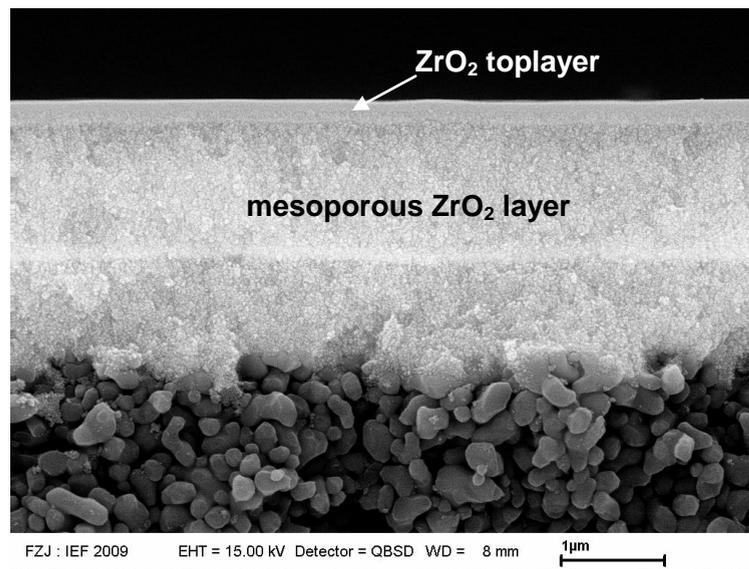
Fig. 2: Microporous ZrO<sub>2</sub> membrane on top layer of a high quality mesoporous ZrO<sub>2</sub> layer
