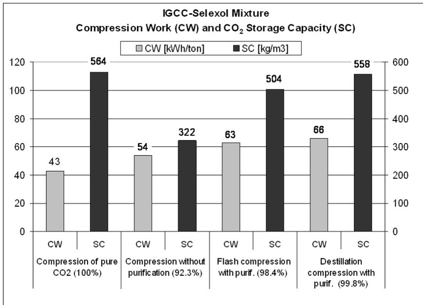
Fig. 11: Compression work and storage capacity for an IGCC-off gas [Castillo 2009]
