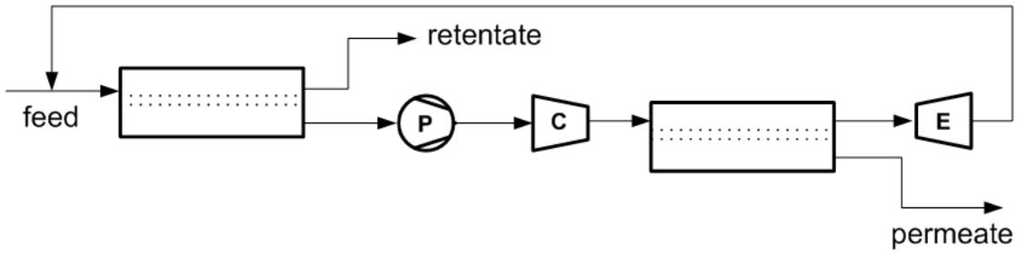
Fig. 7: A cascade concept, recycling the retentate of the 2<sup>nd</sup> membrane to the feed of the 1<sup>st</sup> membrane
