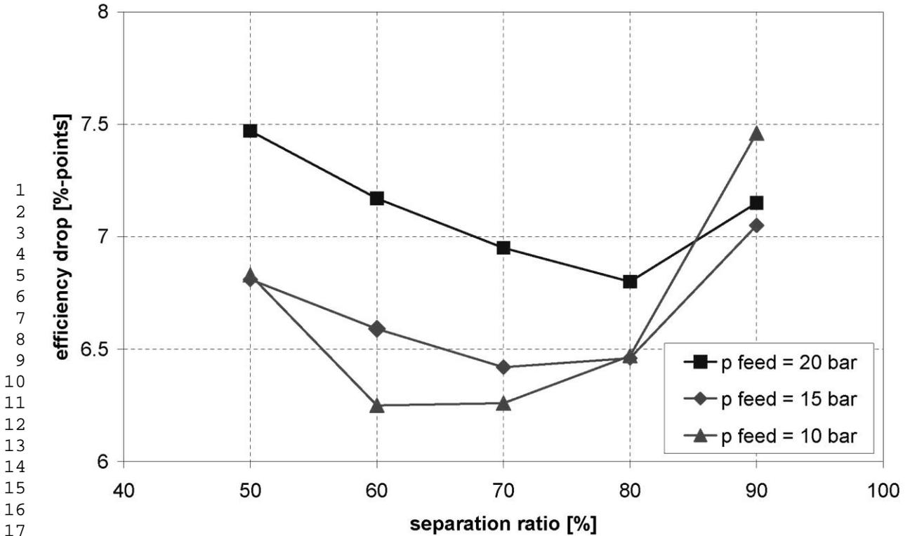
Fig. 10: Efficiency drop of an 3-end oxyfuel power plant at different feed pressures and separation ratios.
