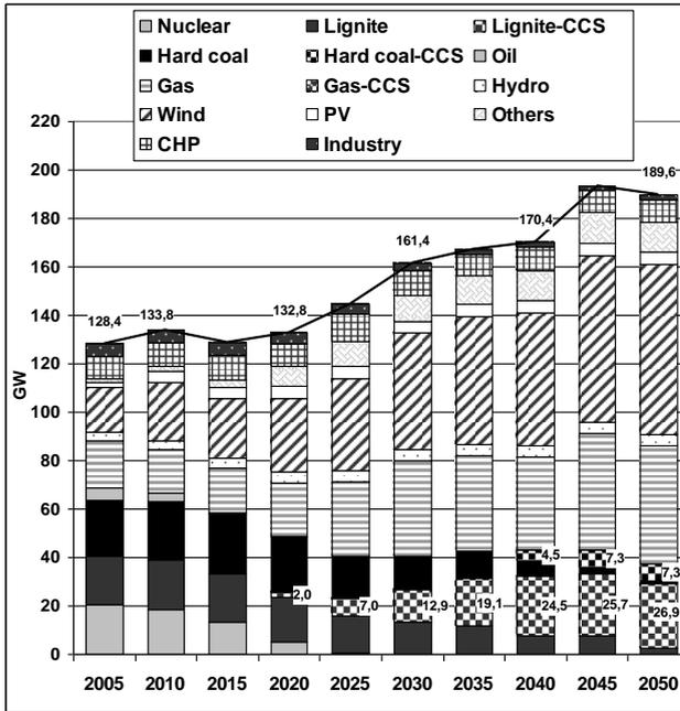
Fig. 14: German power plant capacity meeting a 69 % CO<sub>2</sub> reduction target until 2050
