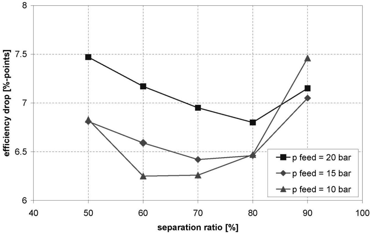
Fig. 10: Efficiency drop of an 3-end oxyfuel power plant at different feed pressures and separation ratios.
