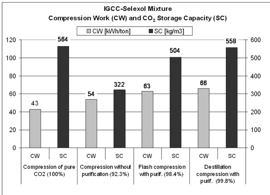
Fig. 11: Compression work and storage capacity for an IGCC-off gas [Castillo 2009]
